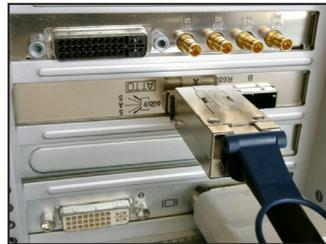
G-SPEED eS Pro is shipped from the factory setup in RAID 0 mode for best performance. The ATTO R680 RAID controller also supports RAID 1, 5, 6 and JBOD modes. If you would like to change the RAID mode, see the next section “OSX RAID Configuration Scripts” to re-configure the RAID mode of the G-SPEED eS Pro. You can also refer to the G-SPEED eS Pro User Manual or the ATTO R680 documentation for more information on changing RAID modes.
