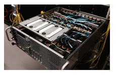
Each custom-designed Netflix video streaming appliance uses 36 6TB HGST Ultrastar He6 drives in a Sanmina chassis.
