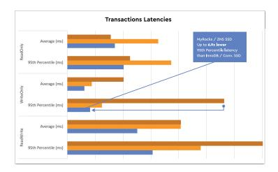
When considering latency in the write heavy scenario, the ZNS SSD equipped server completed the 95% fastest transactions with 6.9x lower latency than InnoDB and with up to 1.5x lower latency than RocksDB in a sever on conventional SSDs.
