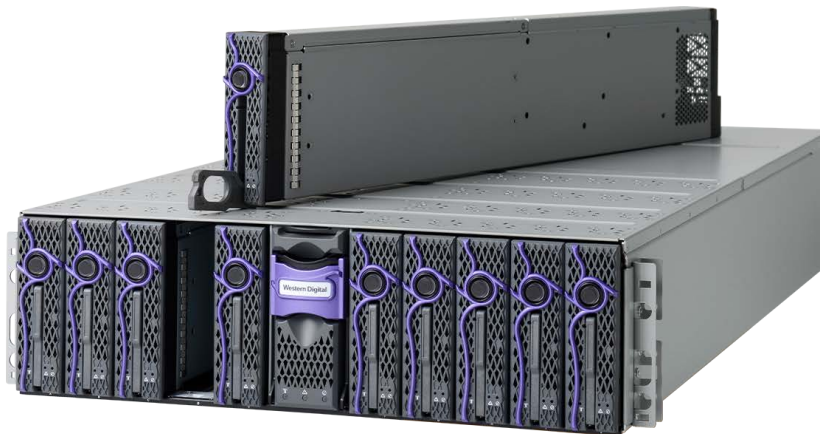
Figure 3-1. OpenFlex™ E3000 enclosure with F3200 Series Fabric Devices
