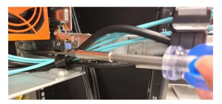
**Step 10:** Install the lower brackets onto the CMA tray.
