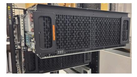
**Step 2:** On the rework unit, move the CMA crossbars and arm(s).
