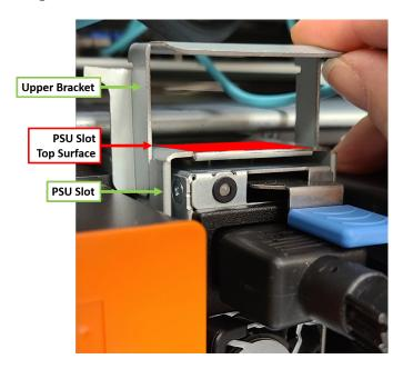
**Step 4:** Remove the backer material from the upper bracket's adhesive film.
