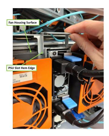
**Step 6:** Slide the bracket down until the adhesive film contacts the top surface of the PSU slot. Press the bracket down to ensure that the adhesive film bonds to the surface.
