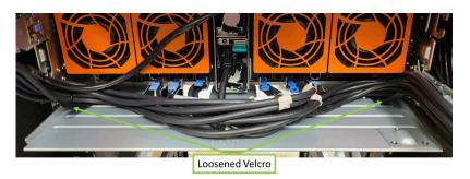
**Step 9:** Remove the CMA tray by loosening its captive screws (x4) using a T15 screwdriver (8" or longer shaft recommended).
