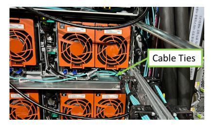
**Step 9:** Remove the CMA tray by loosening its captive screws (x4) using a T15 screwdriver (8" or longer shaft recommended).
