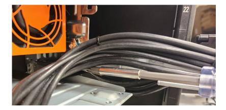
Step 12: Secure the data and power cable(s) to the CMA tray using the hook-and-loop strips.
