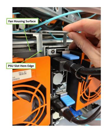
**Step 6:** Slide the bracket down until the adhesive film contacts the top surface of the PSU slot. Press the bracket down to ensure that the adhesive film bonds to the surface.
