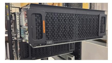
**Step 2:** On the rework unit, move the CMA crossbars and arm(s).
