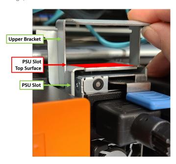
**Step 4:** Remove the backer material from the upper bracket's adhesive film.
