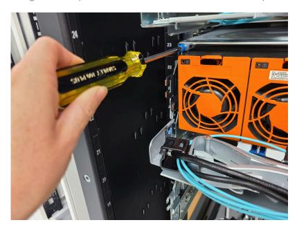
**b.** Swing the CMA crossbar and CMA arm(s) to the side and out of the way.
