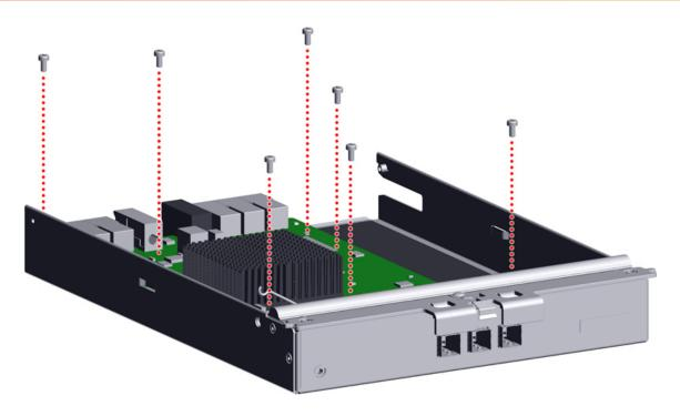
**Step 29:** Pull upward on the circuit board to remove it from the ESM:
