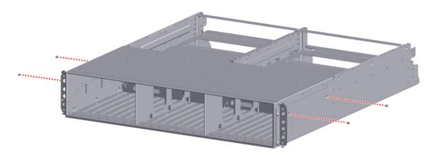
**Step 42:** Using a #2 Phillips screwdriver, remove the four (4) screws on the sides of the chassis, in front of the rack ears:
