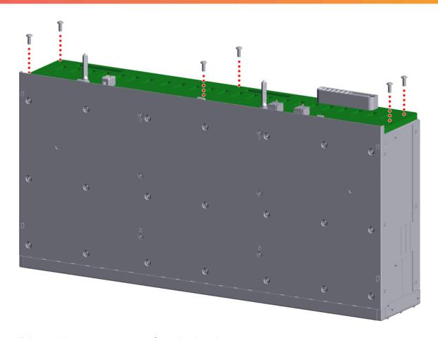
**Step 46:** Pull the midplane up to remove it from the drive housing:
