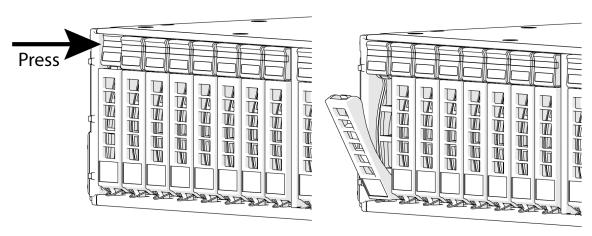
Step 12: Grasp the handle and pull the drive carrier out of the enclosure with even pressure:
