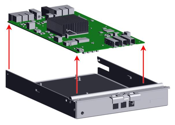
$\textbf{Step 30:} \ \ \text{Repeat these steps to remove the PCB from the remaining ESM}.$
