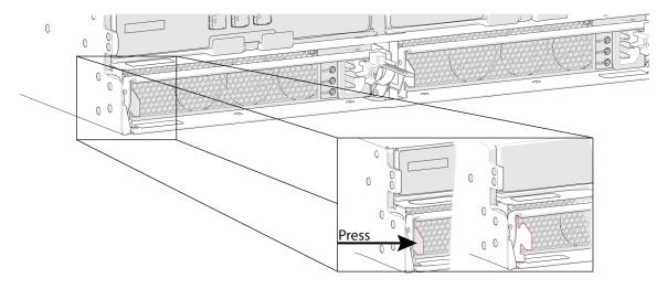
**Step 32:** With the release pressed, swing the handle downward:
