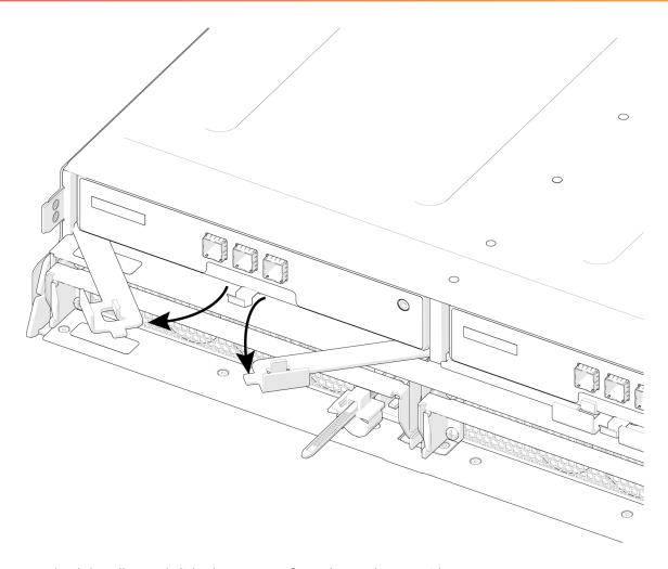
**Step 23:** Grasp both handles and slide the ESM out from the enclosure with even pressure:
