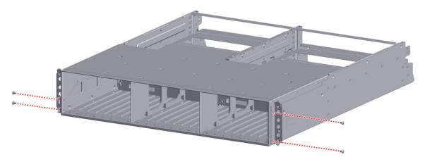
**Step 43:** Pull the drive housing up to remove it from the chassis:
