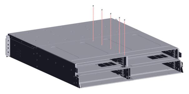
**Step 36:** Using a #2 Phillips screwdriver, remove the six (6) screws on the sides of the chassis, securing the rear cover to the chassis:
