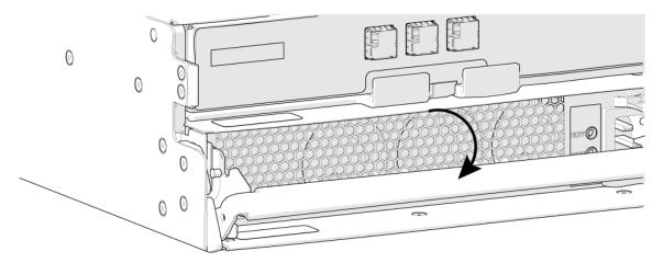
**Step 33:** Use the handle to pull with even pressure and remove the PSU:
