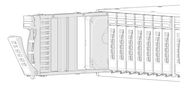
**Step 13:** Repeat these steps to remove the remaining drives from the enclosure. Store each drive assembly in an ESD-safe environment. Do not stack them on top of one another.
