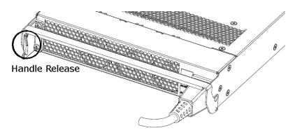
**Step 2:** Detach the cable retention clip from the power cable:
