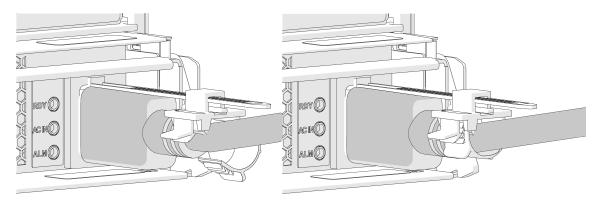
Step 3: Remove the power cable by pulling its plug away from the receptacle on the PSU.
