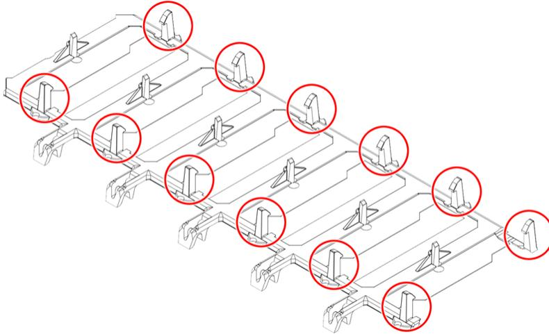
**Step 51:** Use your fingers—or a flat object (flat-head screwdriver, etc.)—to pry up the 10 HDD limiters at their clip locations, and remove the limiters from the baseboard:
