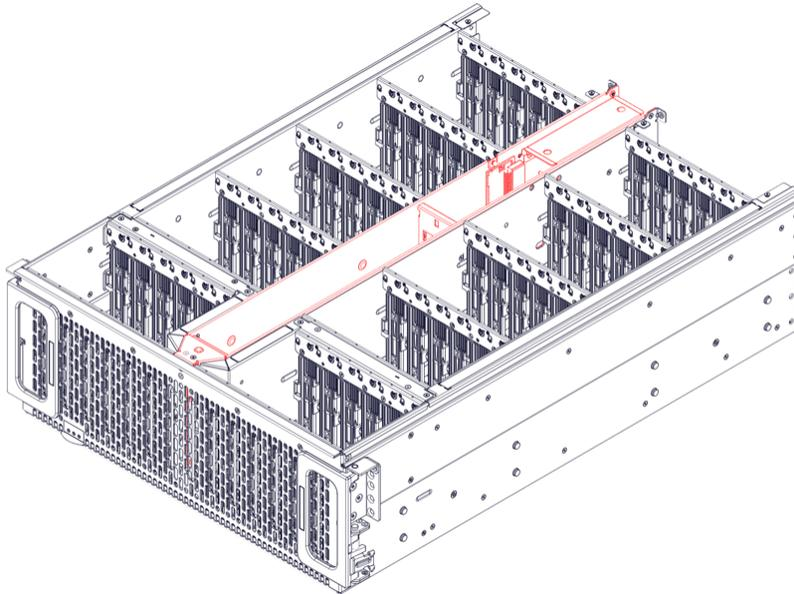
**Step 39:** Use a T7 Torx screwdriver to remove the fourteen (14) M3 6mm screws securing the IO housing to the drive housings and chassis. Then pull the IO housing up to remove it from the chassis:
