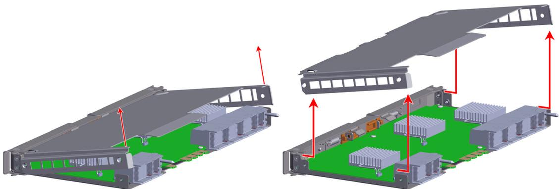
**Step 18:** Using a T10 Torx screwdriver, remove the six (6) M3 4mm pan-head screws securing the circuit board to the other side-panel:
