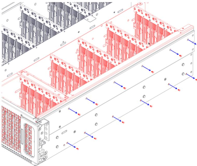
**Step 49:** Pull up on the right drive housing to remove it from the chassis:
