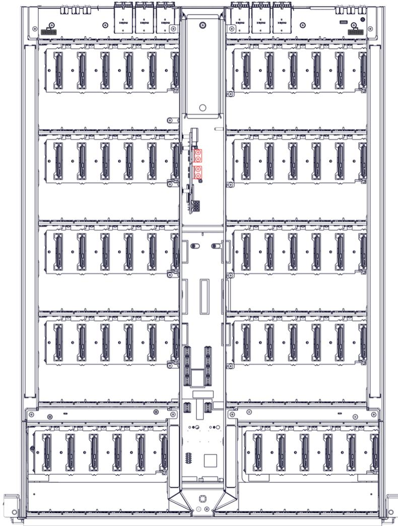
**Step 38:** Use a T8 Torx screwdriver to remove the four (4) M3 6mm screws securing the PDB to the baseboard. The screws are shown in red in the following image:
