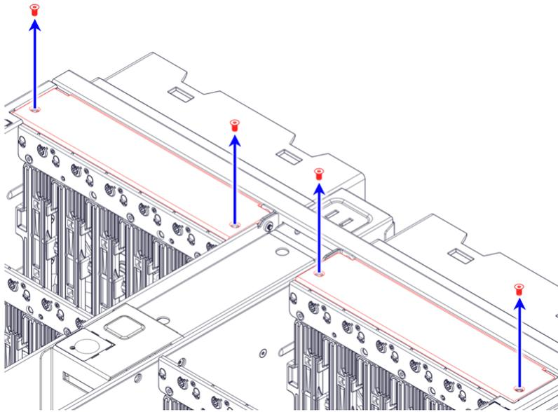
**Step 33:** Pull up on the plenum covers to remove them from the chassis:
