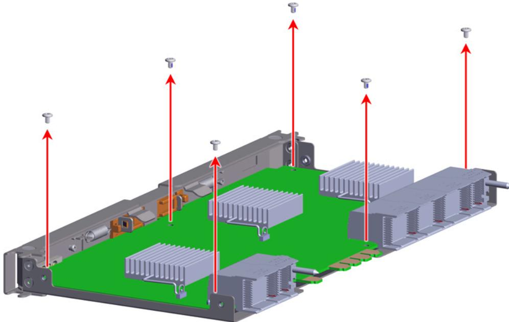
**Step 19:** Pull the circuit board upward to remove it from the IOM:
