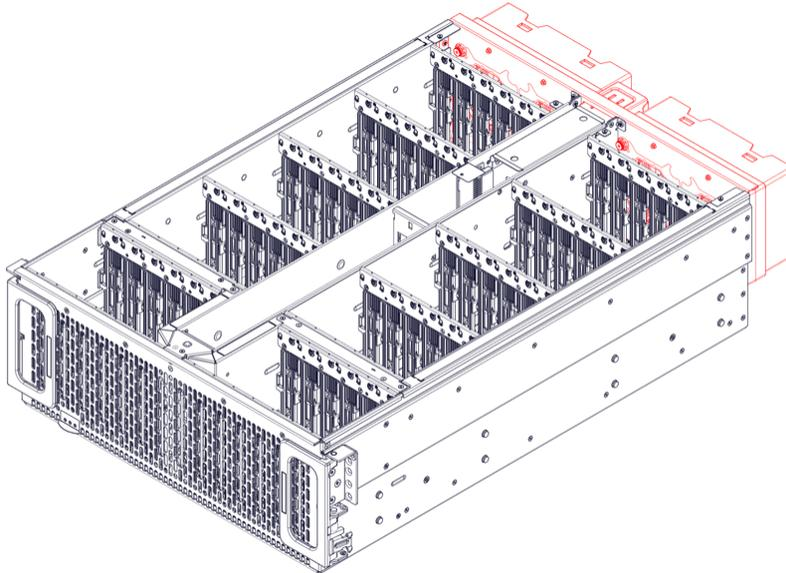
**Step 34:** Use a T7 Torx screwdriver to remove the twelve (12) M3 6mm screws securing the back of the fan housing assembly to the back of the chassis. The screws are shown in red in the following image:
