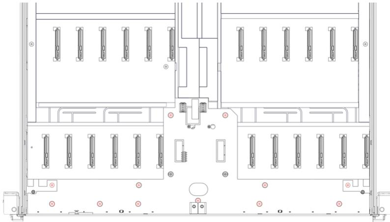
**Step 53:** Pull up to remove the smaller, front baseboard from the chassis:
