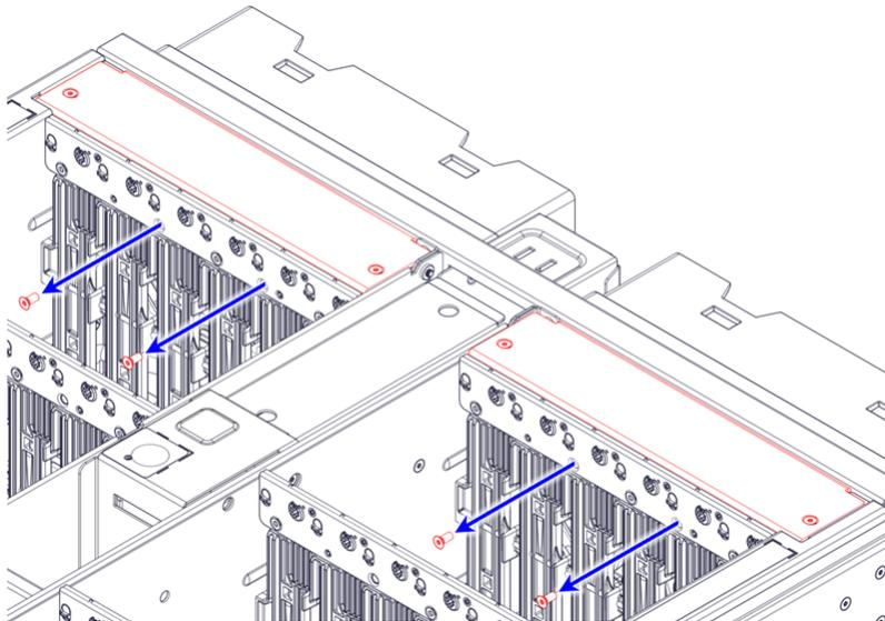
**Step 32:** Remove the four (4) M3 7mm screws securing the plenum covers to the fan housing:
