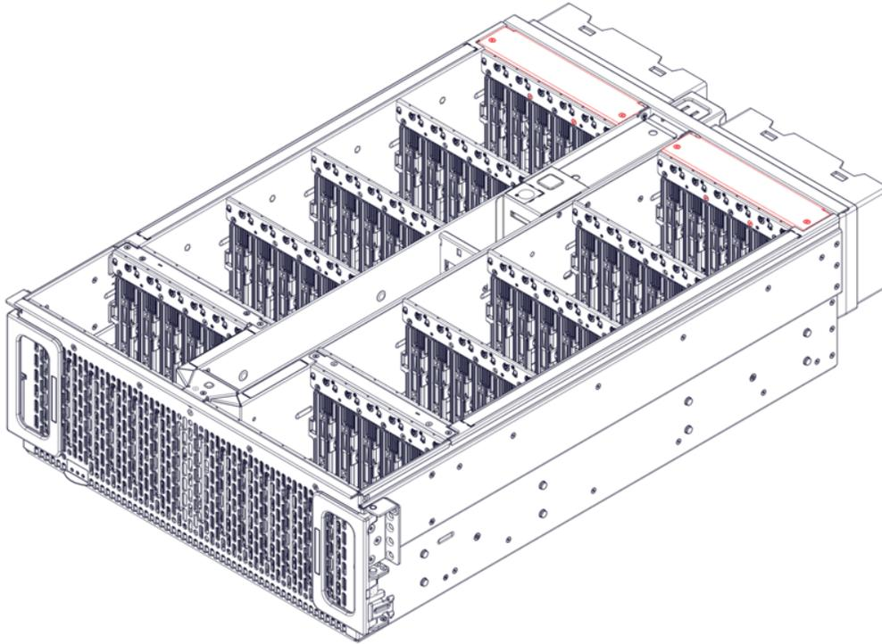
**Step 31:** Use a T7 Torx screwdriver to remove the four (4) M3 6mm screws securing the plenum covers to the left and right drive housings:
