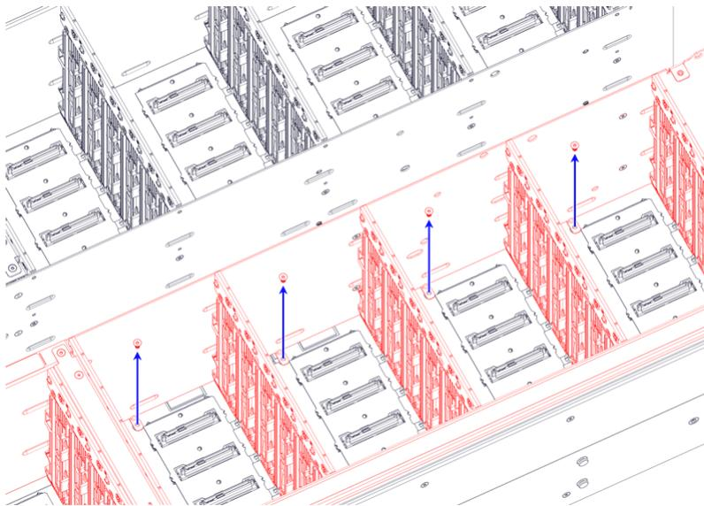
**Step 47:** On the side of the chassis, use a T8 Torx screwdriver to remove the two (2) K30 10mm screws securing the drive housing to the side of the chassis:
