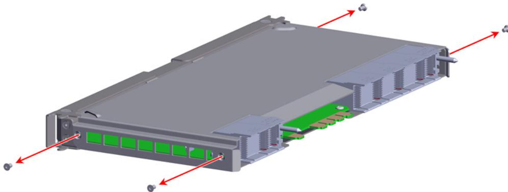
**Step 17:** Lift the bottom edge of the side-panel. Then slide the panel toward the bottom of the IOM before lifting it upward to remove it from the IOM:
