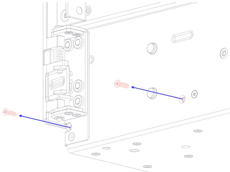
**Step 48:** On the side of the chassis, use a T7 Torx screwdriver to remove the twelve (12) M3 6mm screws securing the drive housing to the side of the chassis:
