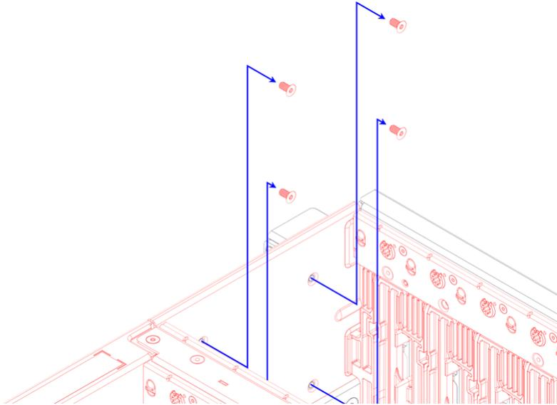
**Step 46:** Inside the drive bays of the right drive housing, use a T7 Torx screwdriver to remove the four (4) M3 6mm screws securing the drive housing to the baseboard:
