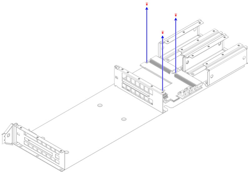
**Step 43:** Lift the PDB to remove it from the IO housing:
