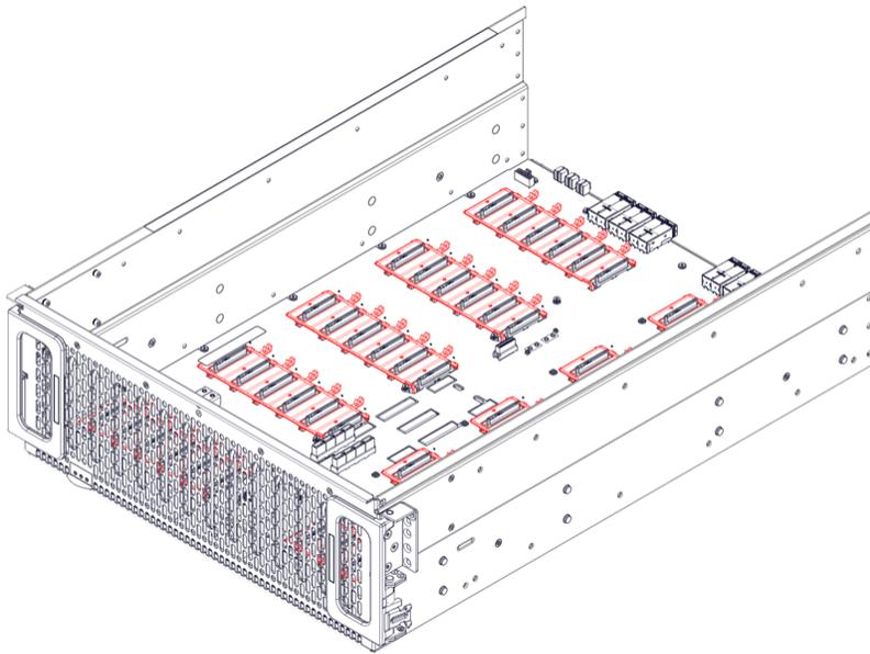
The bottom side of each limiter has twelve (12) clips that hold it to the baseboard; these clips must be disengaged from the baseboard in order to remove the limiter:
