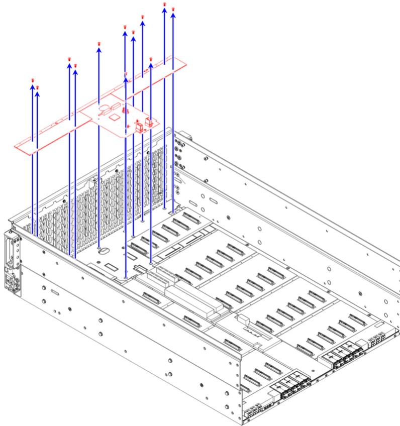
**Step 54:** Use a T7 Torx screwdriver to remove the thirteen (12) M3 6mm screws securing the larger, rear baseboard to the chassis. The screws are shown in red in the following image:
