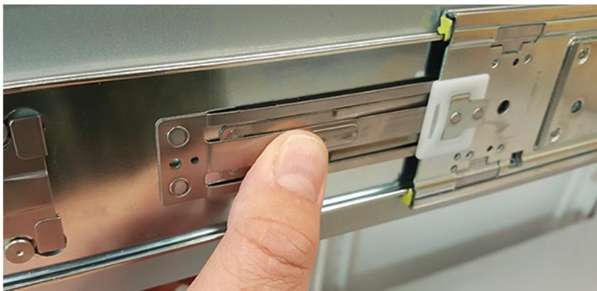
**Step 23:** Push the chassis back into the rack.
