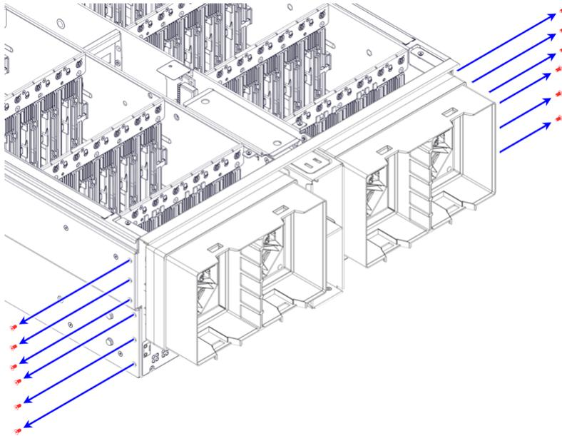
**Step 36:** Pull the fan housing assembly away from the chassis, just far enough to unplug the fan cable connectors from their receptacles on the baseboard. The fan cables, connectors, and receptacles are shown in red in the following image:
