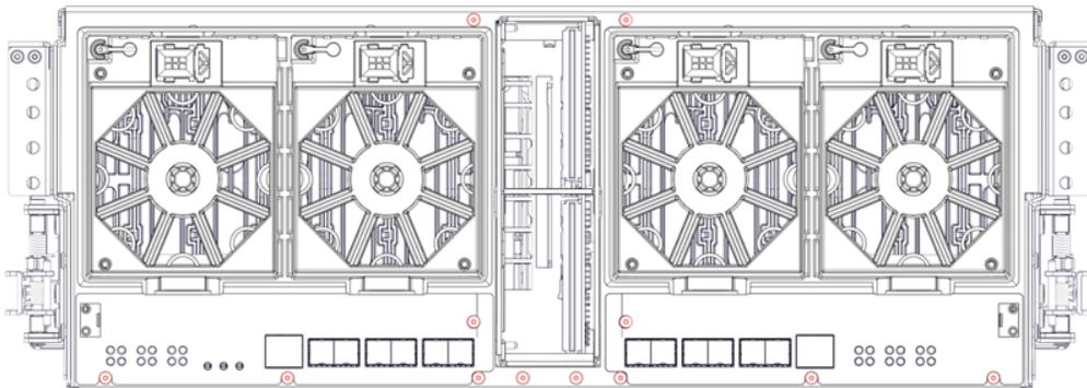
**Step 35:** Use a T7 Torx screwdriver to remove the twelve (12) M3 6mm screws securing the sides of the fan housing assembly to the sides of the chassis:
