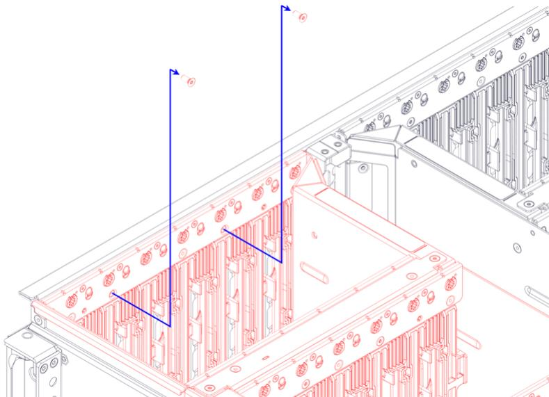
**Step 45:** At the front of the chassis, use a T7 Torx screwdriver to remove the four (4) M3 6mm screws securing the right drive housing to the side of the chassis:
