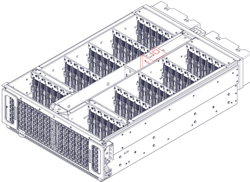
**Step 30:** Use a T7 Torx screwdriver to remove the three (3) M3 6mm screws securing the PDB cover to the left and right drive housings. Then pull up on the PDB cover to remove it from the chassis:
