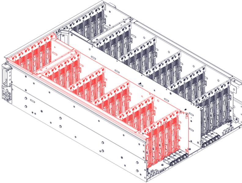
**Step 44:** At the front of the chassis, use a T7 Torx screwdriver to remove the two (2) M3 7mm screws securing the right drive housing to the front of the chassis:
