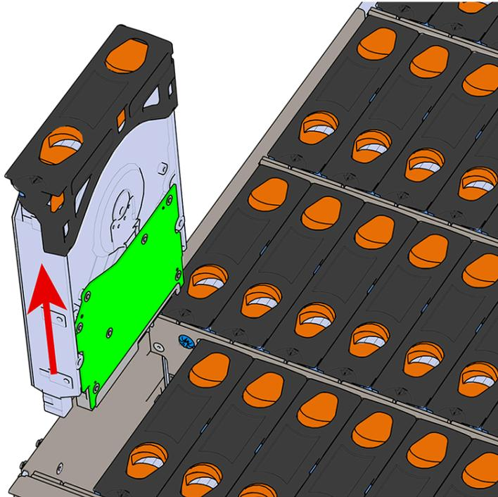
**Step 12:** Repeat these steps to remove all the drive assemblies from the enclosure.
