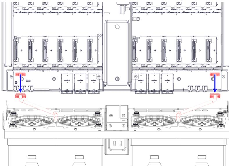
**Step 37:** Remove the fan housing assembly from the chassis:
