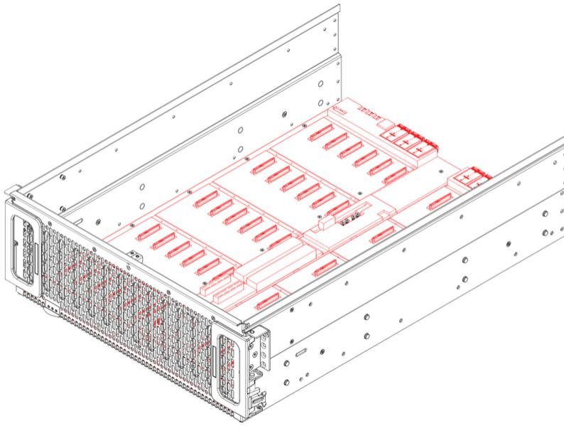
**Step 52:** Use a T7 Torx screwdriver to remove the twelve (12) M3 6mm screws securing the smaller, front baseboard to the chassis. The screws are shown in red in the following image:
