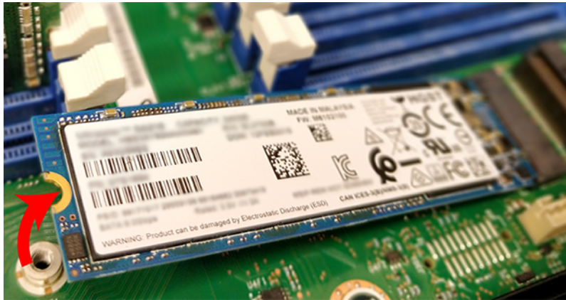
Figure 29: Uninstalling the M.2s
