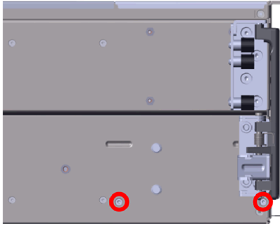
Figure 55: Left Drive Cage T8 Screw Location (Outside of the Chassis)
