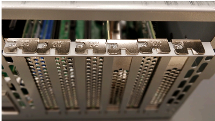
Figure 32: Add-In Card Bracket Removed
