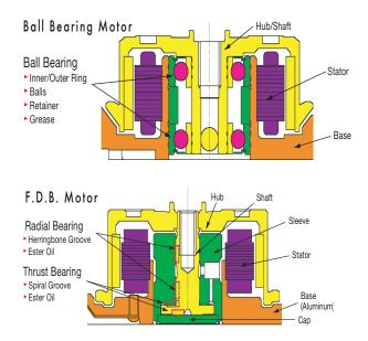
compound the issues of NRRO. Incorporating FBD motors in the design of desktop and mobile hard drives solves many of the issues of NRRO.
