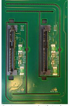
The slots in the baseboard make it act as a suspension that reduces the transmission of vibrations from drives in the arrays, particularly between adjacent drives, by isolating the motion of the drives. The Ultrastar platform also uses vibration isolated fans to minimize this source of vibration. ArticFlow also reduces the vibration in the system by enabling the use of lower fan speeds, so the fans generate less vibration, and a side benefit is they use less power to cool the storage system.
