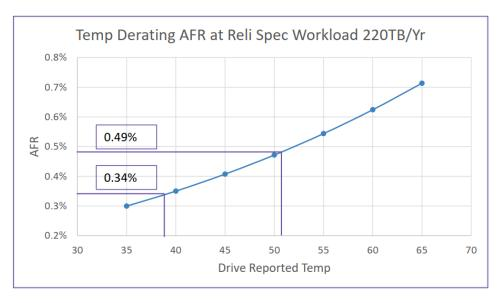
As shown on this graph, as the HDD temperature increases, the expected AFR of a collection of HDDs operating at this temperature increases.
