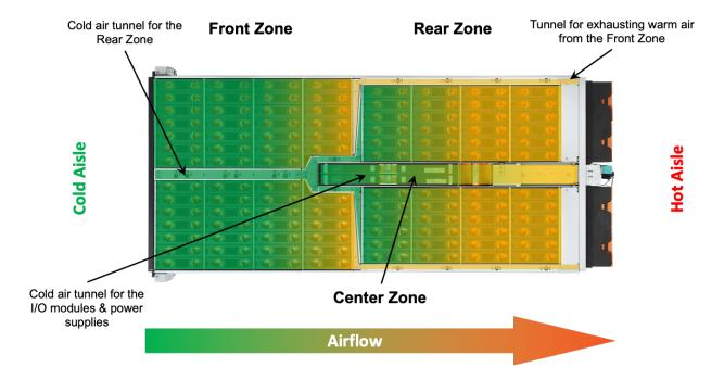
Warmed air from the first zone is ducted away from the second zone so the second zone drives aren't heated by that warm air. Cool air is drawn into the center of the enclosure from the cold aisle to cool the second zone HDDs. As a consequence of having two HDD cooling zones, overall HDD temperatures are cooler and more uniform leading to lower HDD failure rates. There is also a dedicated third cooling zone to channel fresh air to the I/O modules and power supplies.
