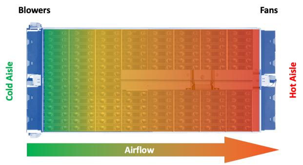
With blowers to push air into the storage shelf from the cold aisle and fans to pull the air out of the shelves into the hot aisle, the drives nearest to the blowers stay cooler, but the drives farther from the blowers get hotter as the air flowing through the shelf gets hotter and don't pull as much heat from the HDDs.
