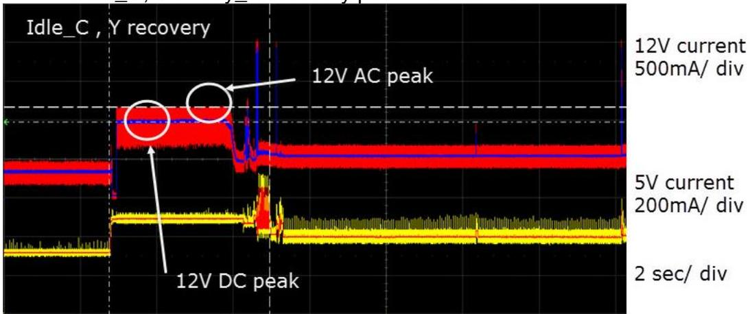
Figure 7 Idle\_C Standby\_Y recovery current waveform
