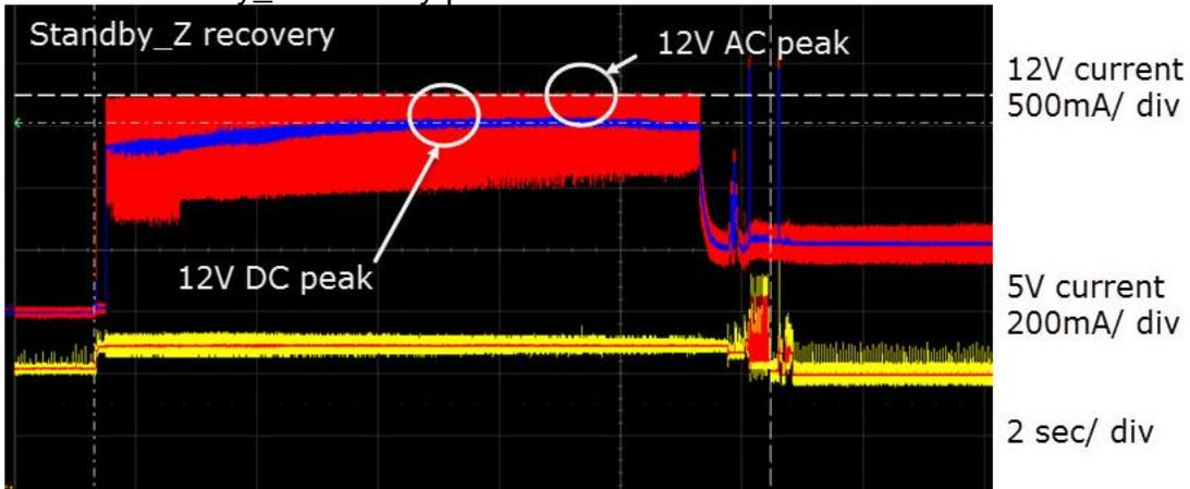
Figure 8 Standby\_Z recovery current waveform
