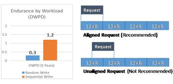
Ultrastar DC SN340 requires requests be 32KB aligned. For other alignments, Ultrastar DC SN640 may be a more suitable option.
