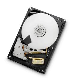
The Deskstar 7K4000 & Deskstar 5K4000 hard drives feature Advanced Format technology. Advanced Format increases the physical sector size on hard drives from 512 bytes to 4096 (4K) bytes, which increases drive capacities and improves error correction capabilities. Please consult the HGST Advanced Format Drives page for more information on using these hard drives.
