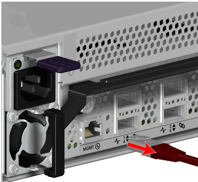
**Step 8:** Repeat the previous step to uninstall the remaining Ethernet cable.
