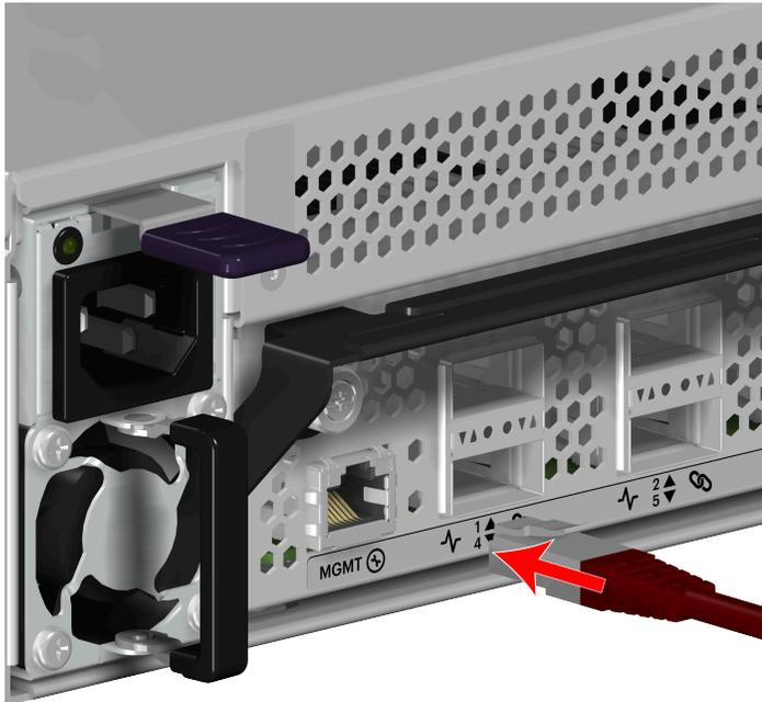
**Step 17:** Repeat the previous step to install the remaining Ethernet cable.
