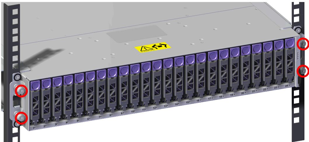
Figure 118: Captive Screw Loosen
