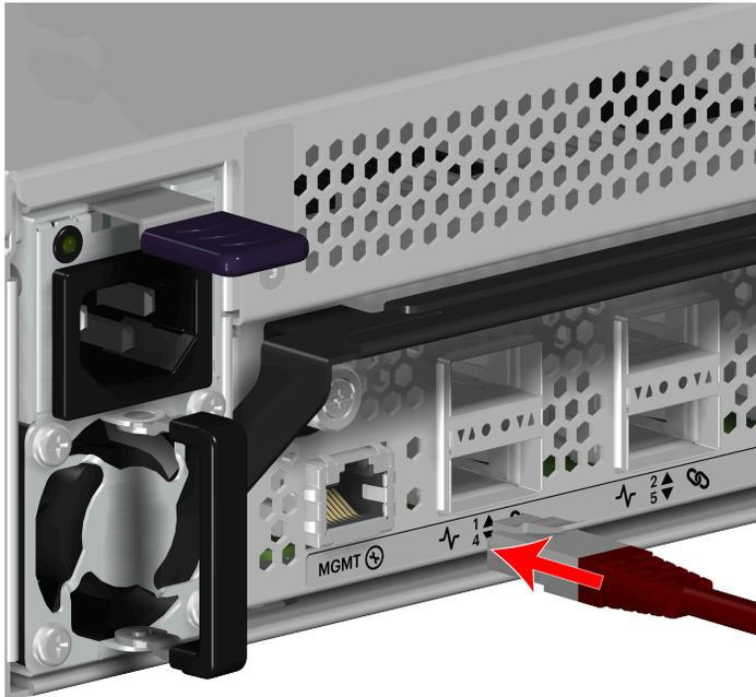
**Step 28:** Repeat the previous step to install the remaining Ethernet cable.
