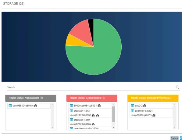
The **Storage Health** modal provides an overview of the health of all storage devices visible on the fabric (those in the subnets of what is configured on the enclosure). The modal provides separate tables for fabric devices that are presenting different health states up to the OCGUI.
