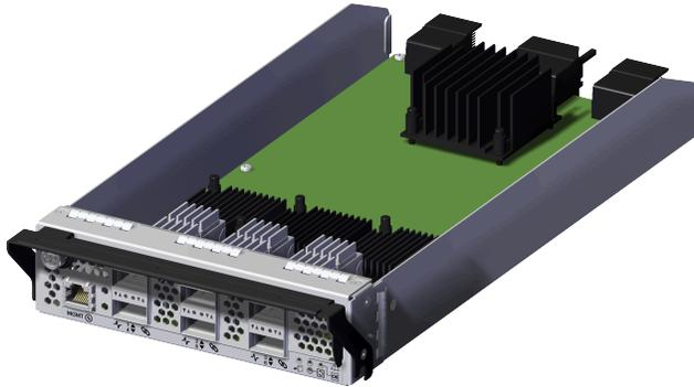
Each IOM contains three, chip down RapidFlex A2000s that provide system data connectivity through a QSFP28 cable, and supports cable lengths up to 10m. Out-of-Band Management (OOBM) features are accessed via an RJ45 port that supports a 10/100/1000 Mbps Ethernet connection. The IOM status LEDs report Fault and Power. The IOM is hotswappable and easily removable by removing cables/connectors, loosening the single thumbscrew and pulling on the handle.
