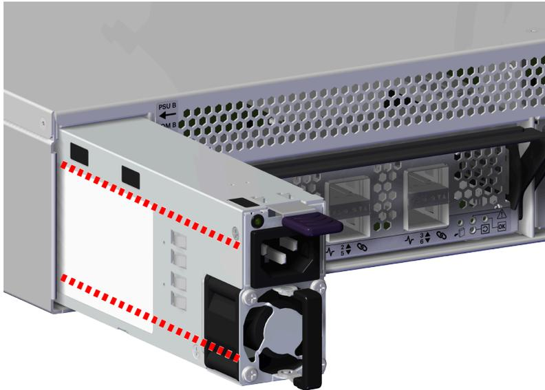
**Step 12:** Repeat the previous step to uninstall the remaining PSU.
