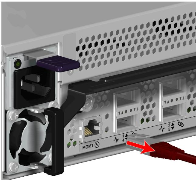
**Step 7:** Repeat the previous step to uninstall the remaining Ethernet cable.
