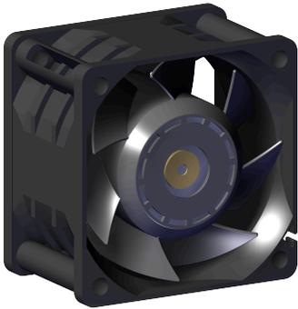
The System Fans provide the primary system cooling for the OpenFlex Data24 4000 Series. There are a total of four N+2 redundant fans. The System Fans are coldswap capable components, and require the system to be shut down for servicing and accessed by removing the chassis cover.
