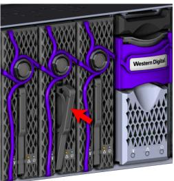
**e.** Verify that the F3x00 is securely latched into the chassis by pulling on the latch and ensuring the device does not move when pulled. Reinstall the device if it is not securely installed into the chassis.
