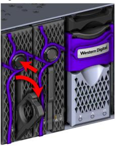
**b.** Use the release handle to pull the device blank out of the enclosure part way. Then grasp the device blank from the underside to support it as you pull it the rest of the way out of the enclosure.
