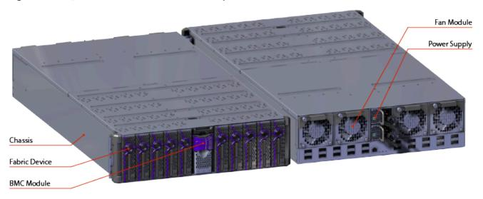
The enclosure measures 447.2 mm/17.6 in. wide by 828.04 mm/32.6 in. long. It's height is 130.9 mm/5.2 in. or 3U. The chassis installation length is 778 mm (30.6 in.) from front rack chassis mounts to rear of system.
