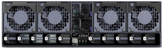
**b.** Press the release button on the front of the OpenFlex F3x00 . The release handle will eject outward.
