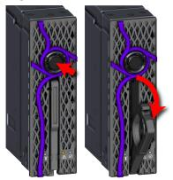
**b.** Use the release handle to pull the OpenFlex F3x00 out of the enclosure part way. Then grasp the OpenFlex F3x00 from the underside to support it as you pull it the rest of the way out of the enclosure. See the hand placement in the image.
