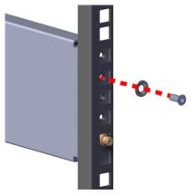
**c.** Remove the rails from the rack by sliding the rail mounts out of the vertical rack rail. The rail uses a spring loaded mechanism to secure the rails into the rack before securing them with the provided screws.
