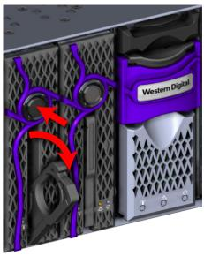
**b.** Use the release handle to pull the OpenFlex F3x00 out of the enclosure part way. Then grasp the OpenFlex F3x00 from the underside to support it as you pull it the rest of the way out of the enclosure. See the hand placement in the image.
