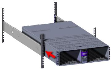
**b.** Use a T15 Torx screwdriver to install three M5 screws in each rack ear (6 total), securing the chassis to the vertical rack rails:
