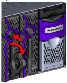
**b.** Use the release handle to pull the device blank out of the enclosure part way. Then grasp the device blank from the underside to support it as you pull it the rest of the way out of the enclosure.
