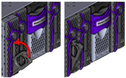
**d.** Rotate the release handle up and press it into the OpenFlex F3x00 to secure it into the slot. When it is fully installed the user will feel the handle snap and lock into place.
