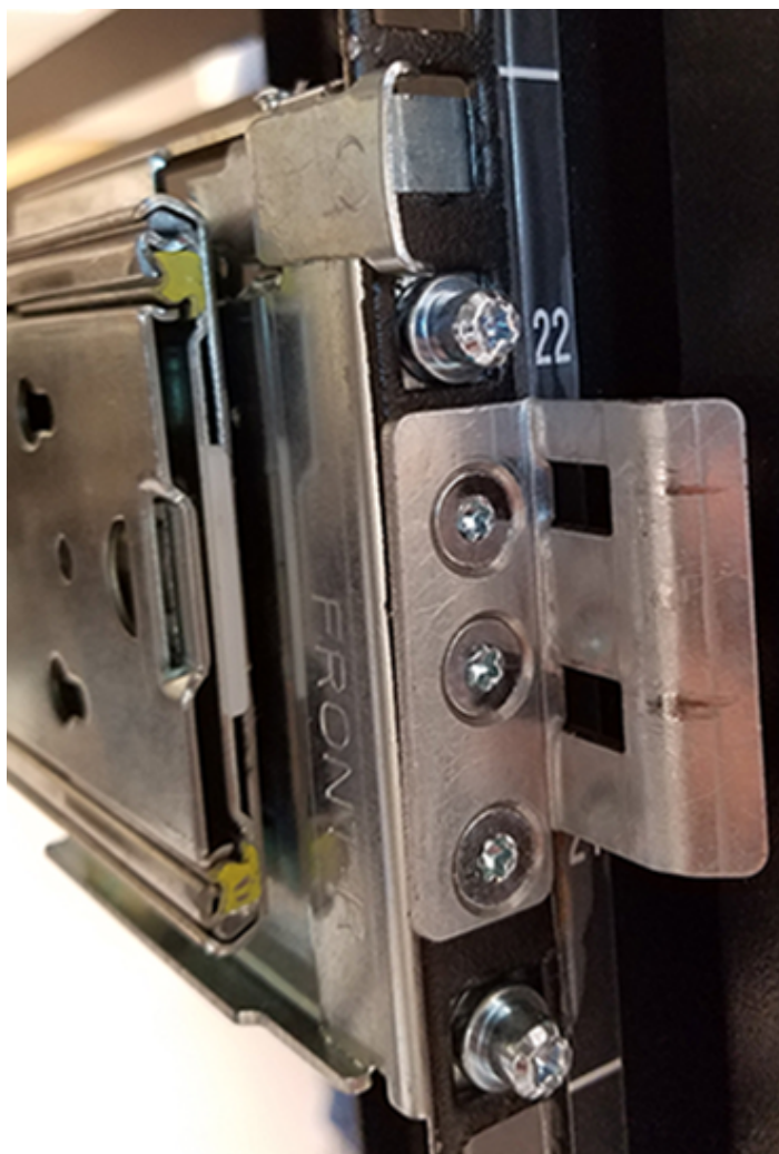
Figure 29: Rack Latch Bracket Installed
