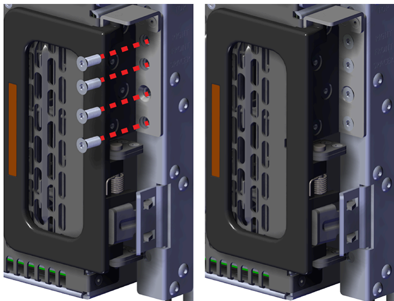
Figure 67: Shipping Bracket Screw Locations (CMA Lite)
