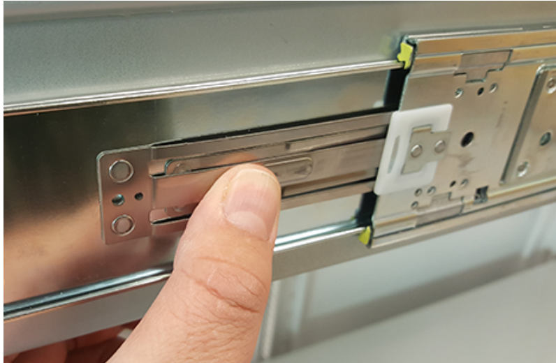
Figure 81: Safety Latch Release
