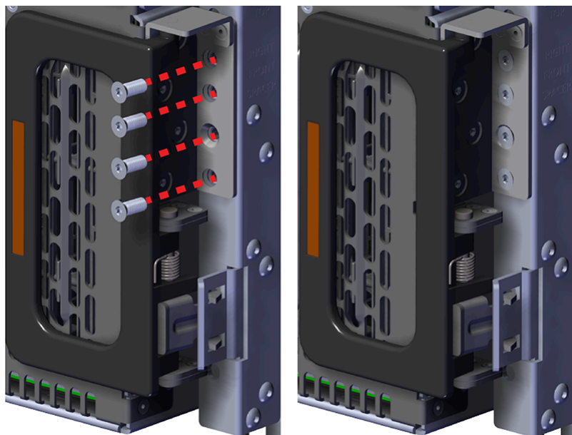
Figure 144: Shipping Bracket Screw Locations (CMA Lite)
