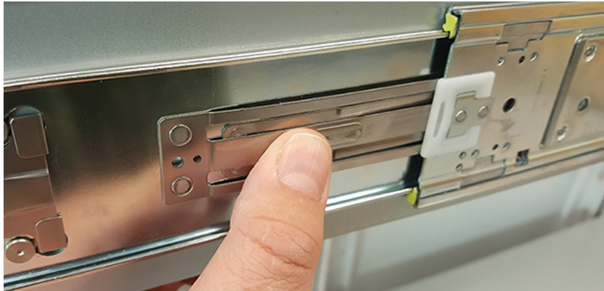
Figure 80: Inner Rail Safety Latch Release
