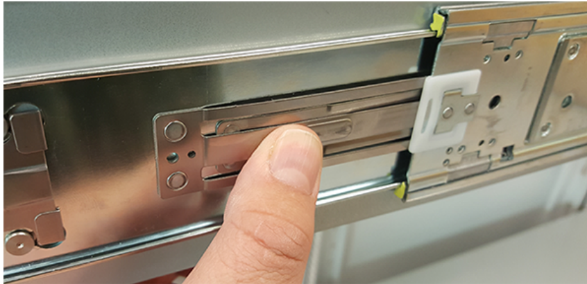
Figure 120: Inner Rail Safety Latch Release
