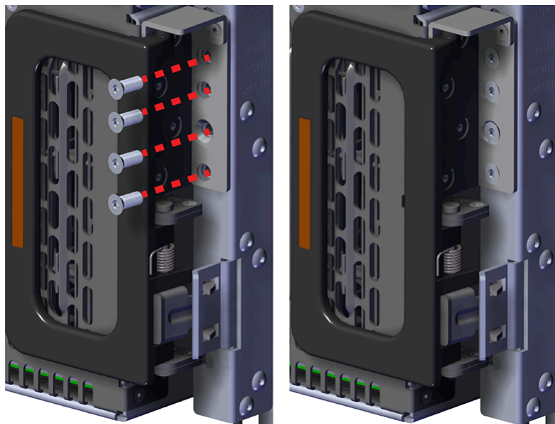
Figure 209: Shipping Bracket Screw Locations (CMA Lite)
