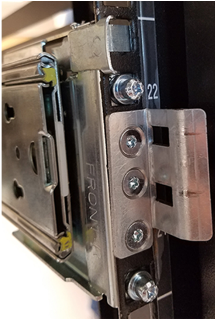
Figure 138: Rack Latch Bracket Installed
