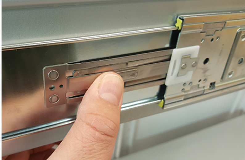
Figure 122: Safety Latch Release
