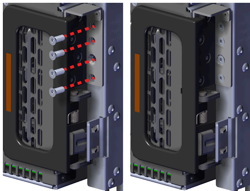
Figure 110: Shipping Bracket Screw Locations (CMA Lite)
