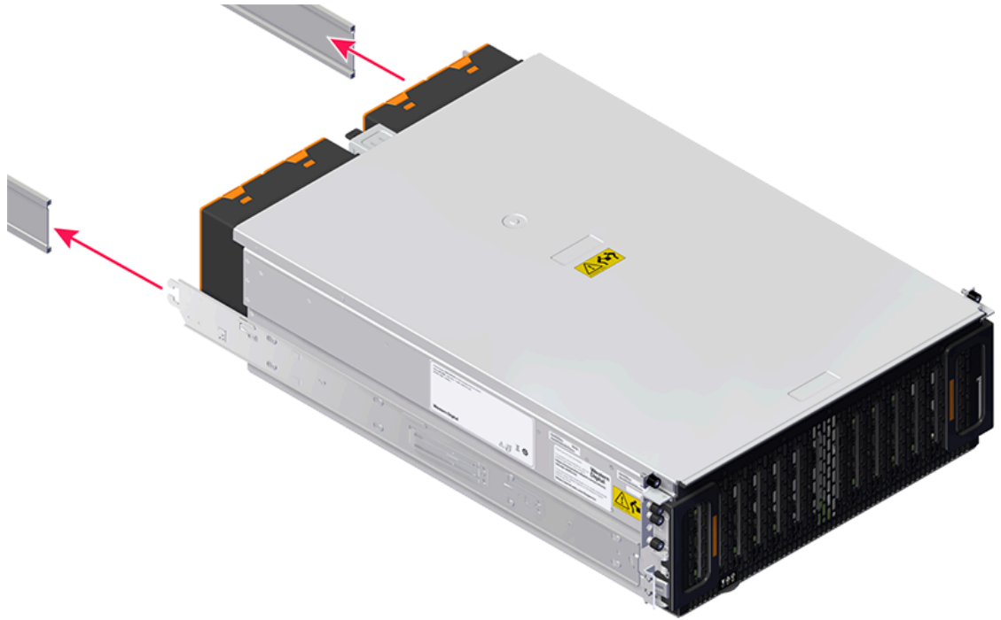
Figure 28: Install the Chassis Into the Rack
