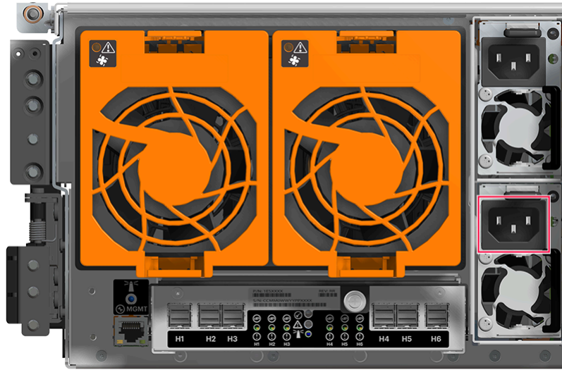
Figure 60: Install the Lower PSU Cable
