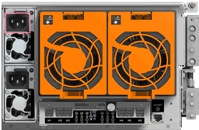
Figure 65: Install the Upper PSU Cable
