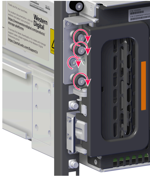
Figure 74: Tighten the Rack-Ear Screws
