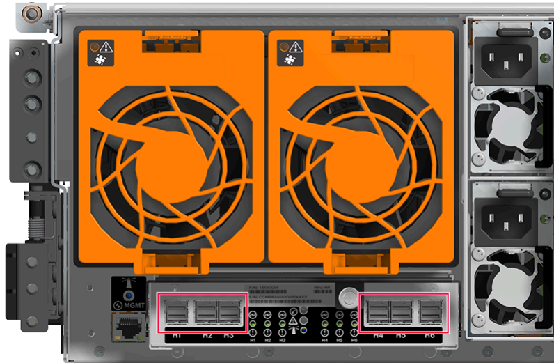
Figure 59: Install the Left SAS Cables
