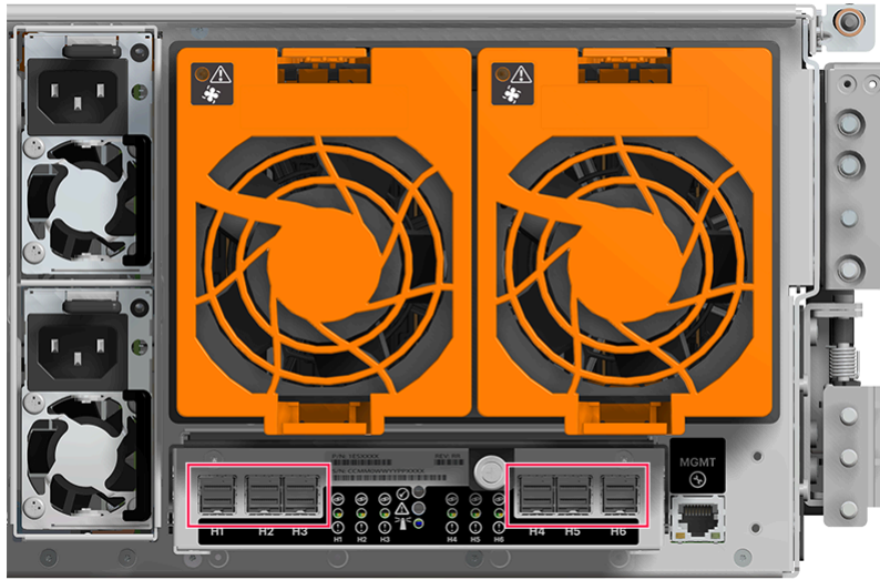
Figure 64: Install the Right SAS Cables
