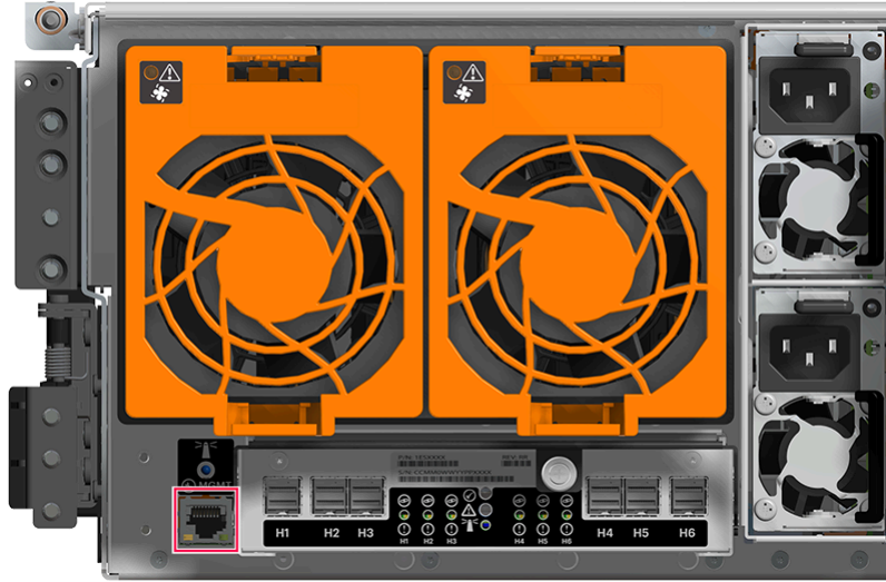
Figure 58: Install the Left Management Cable
